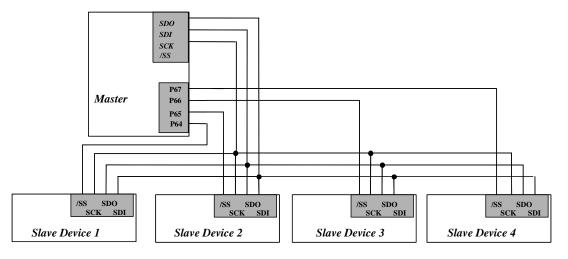
Fig. 18. The SPI Configuration Example of Single-Master and Multi-Slaves
